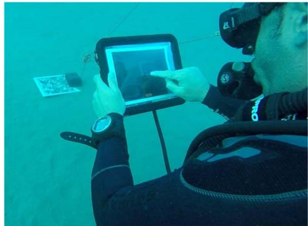
Figure 3 Underwater tablet and housing
